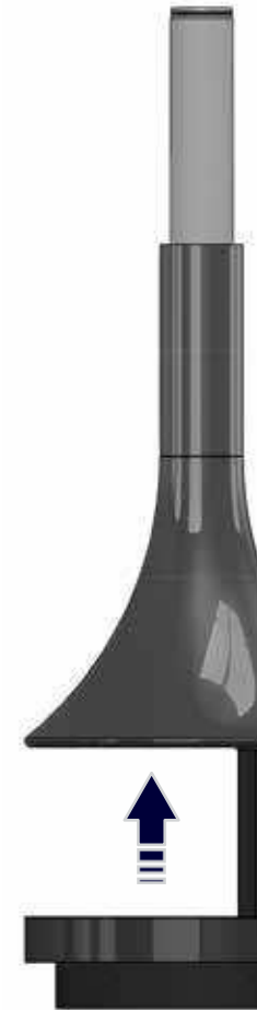
Raise the vent pipe back into place.
