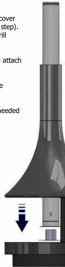
Attach the vent pipe to the large ring.
