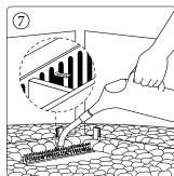
Always fill the burner only with the amount of "Bio-Fuel" required for the desired burn period (consumption rate is approx. 500 ml/h)! Please follow the indicated safety recommendations and warning notices!
