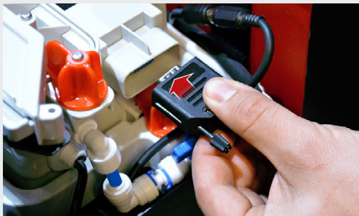
130 Plug in the plug for the control cable again.
