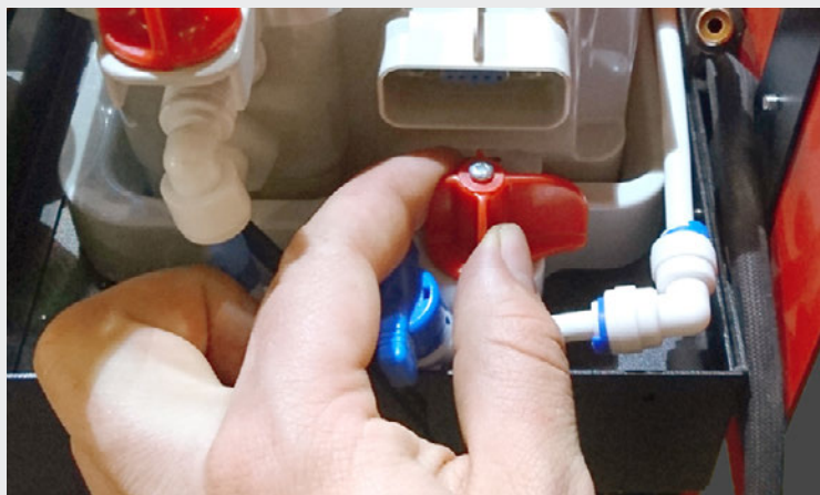
116 Now turn the two lower, side, red handles (left and right on the sump holder) outside around the sump.
