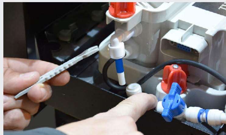
119 The piping unit inlet is now separated from the sump.
