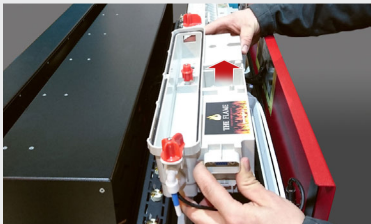
14 Now the sump can be lifted up from the burner.
