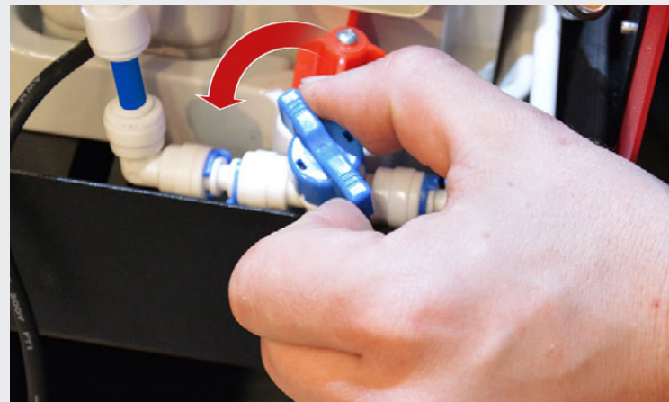
129 Open the Bio-Fluid-cable valve with a turn against clock-wise for 90°.
