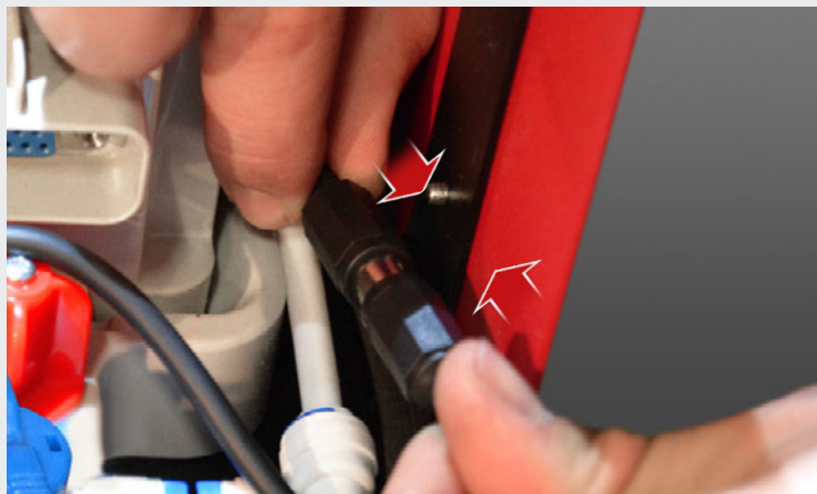
128 Plug the Cinch-plug again in the sensor line.
