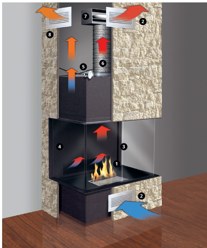
BIT WITH INDOOR EXHAUST AIR
