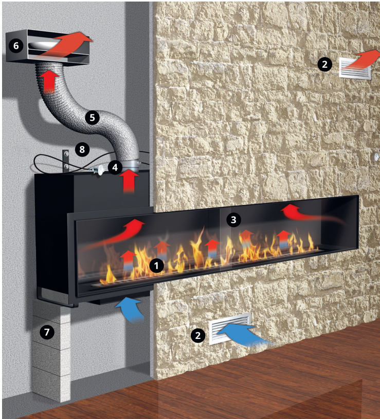
GAP WITH INDOOR EXHAUST AIR
